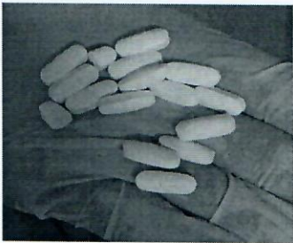
Gambar 3. Kaplet Patah Hasil Friability
