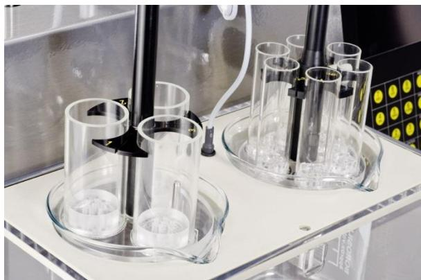
The built-in heating system of the PTZ AUTO EZ instrument uses a silent circulation pump and a heater to pre-heat the outer water and keep the temperature within a tight tolerance. The actual bath temperature is displayed at all times and measured by an external movable temperature probe inside the water bath. The overheating protection system includes a pressure gauge to monitor the pump flow, a thermo switch and thermo fuse to cut the power supply in case of an electronical fault.
