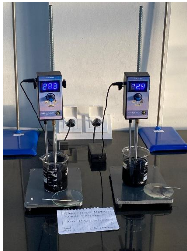
Gambar 3.2 Proses adsorpsi sistem batch
